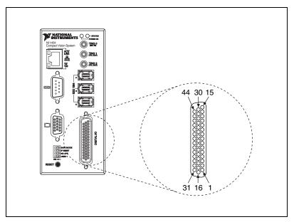
Figure 3-8. 44-Pin DSUB Connector
